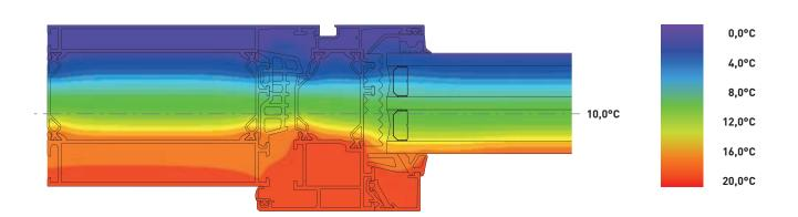
Isothermal curve in line with U<sub>r</sub> EN ISO 10077-2
