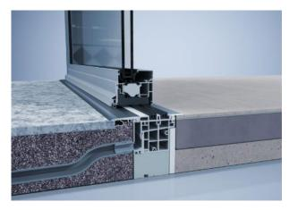
The flush ground threshold contains two magnetic profiles embedded in the frame that are automatically raised when closing. This creates a perfectly tight seal when the element is closed. © heroal
