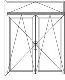
A tilt casement and two pivoting / tilt casements
